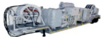
Trailer Mounted Substation
